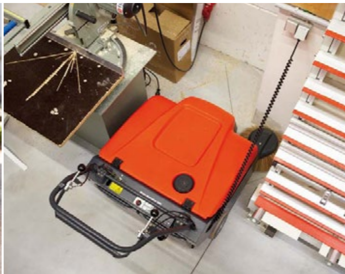
DustStop(option) reduces dust and fine particulate emissions at the side broom by up to 90%.
